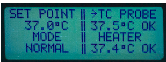
Fig. 7—The home page display shows the set point, mode, control temperature and plate temperature.
