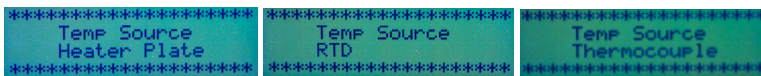
Fig. 8—One of three source temperatures can be used to control the animal's temperature.
